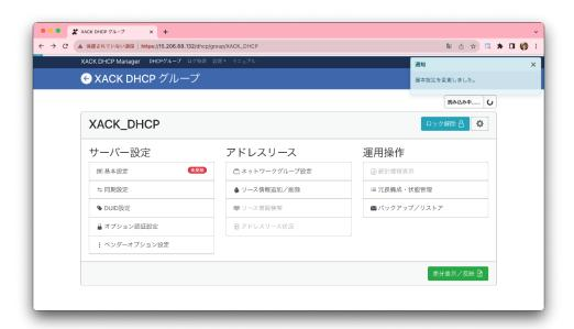
I return to the "XACK DHCP Group" screen, but "Basic Settings" is displayed as "Not Reflected" in red due to pressing the [Save] button earlier. The current state is that the settings have been made on the GUI (XACK DHCP Manager) side, but they have not been reflected in the DHCP server (XACK DHCP).
