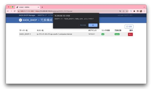
If "Server XACK\_ DHCP-1 has been stopped" appears in the upper right corner, the server has been stopped successfully.
